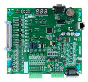
Hardware configuration: 24-way digital input, 6-point relay output, strong current detection terminal, analog differential input, 485 differential signal, RS232, dedicated to synchronous machine.
