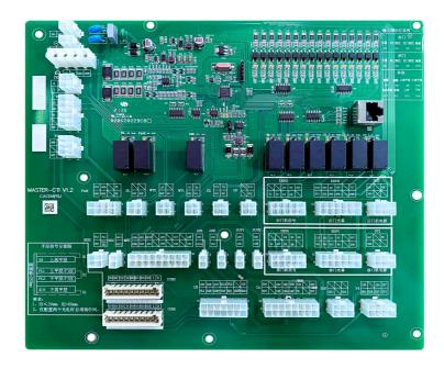
Hardware configuration: 16 digital inputs, 9 relay outputs, 1 analog input, 1 CAN communication.
