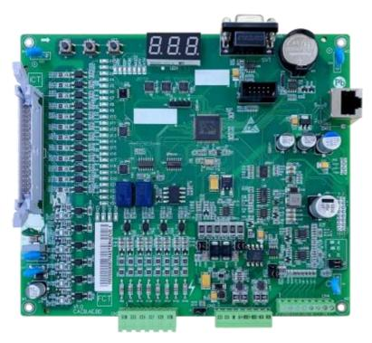
Hardware configuration: 24-way digital input, 6-point relay output, strong current detection terminal, analog differential input, 485 differential signal, RS232, dedicated to asynchronous machines.
